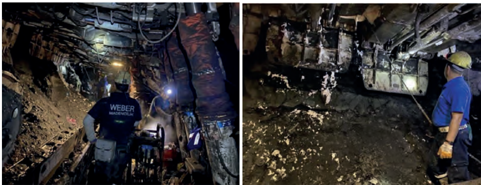
Figure 1. Cavity in longwall mining.
