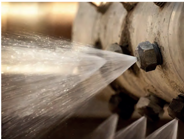
Figure 6. Misting heads differ from spray bars, in that a large number of nozzles can be mounted at various angles for better coverage.
