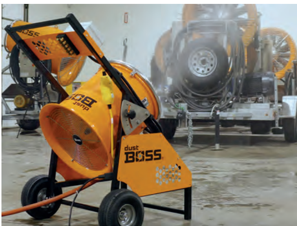
Figure 7. Smaller cannons can be mounted in loading and discharge zones to improve workplace air quality.
