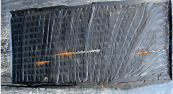
Figure 2. Visually undetectable rope corrosion in the conveyor belt.
