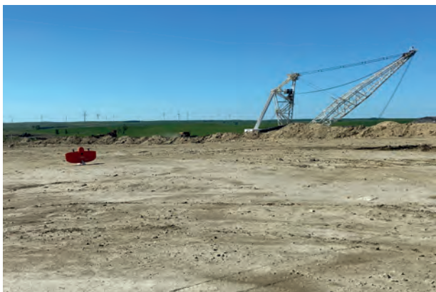
Figure 2. BNI's 8200 dragline strips 40 000 – 60 000 yds of earth (3 – 5 ha.) a day, so regular drone surveys are a boon for tracking progress and keeping records.
