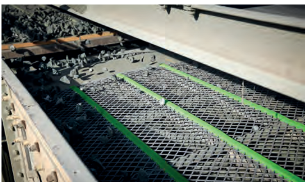
Figure 3. The inclusion of polyurethane strips within the design of high-vibration wire screen media boosts its durability, without sacrificing open area.
