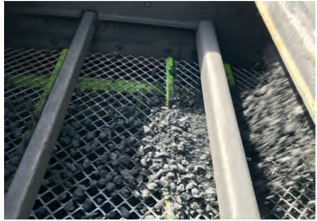
Figure 4. High-vibration panels can withstand harsher screening conditions with the most abrasive materials, such as granite and basalt.
