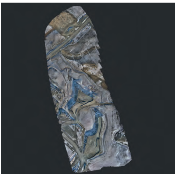
Figure 3. BNI Coal maps gravel stockpiles with WingtraOne and its Sony RX1R II payload covering 81.4 ha. (201 acres) in 42 min., at a GSD of 1.61 cm/0.63 in. This pushes analytics and site planning to a new level of functionality.
