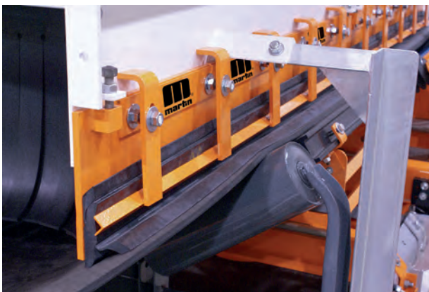
Figure 7. The raised skirtboard allows room for the external wearliner to perform its function and be changed easily from outside the system.
