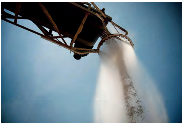
Figure 3. A dust ring suppresses dust from the discharge point to the top of the pile.
