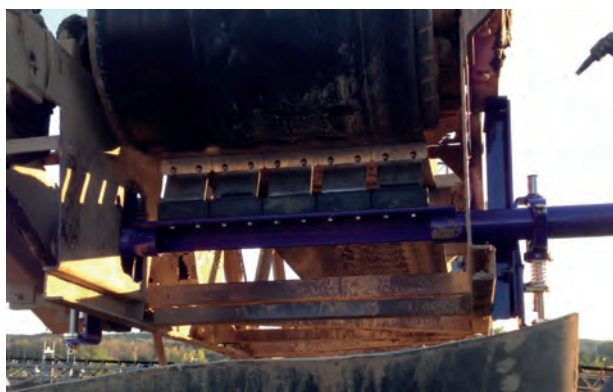
Figure 2. Over time, a belt that has been maintained with a secondary cleaner will last longer.
