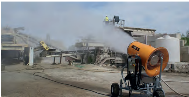
Figure 2. Upwind wide-area dust control can help operators reduce emissions by introducing millions of droplets.
