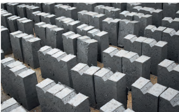
Figure 2. Blocks of fly ash bricks drying at manufacturing site.
